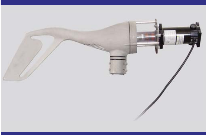
The Wind Turbine Generator with DC Motor is comprised of a 90VDC permanent-magnet type 1800 rpm for mounting to the wind turbine shaft in order to simulate wind energy. A 180VDC version of this model is also available.
