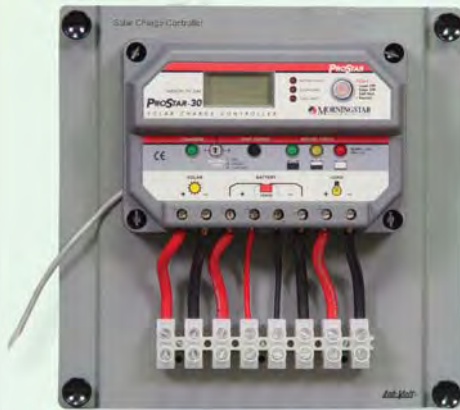
Solar Charge Controller
