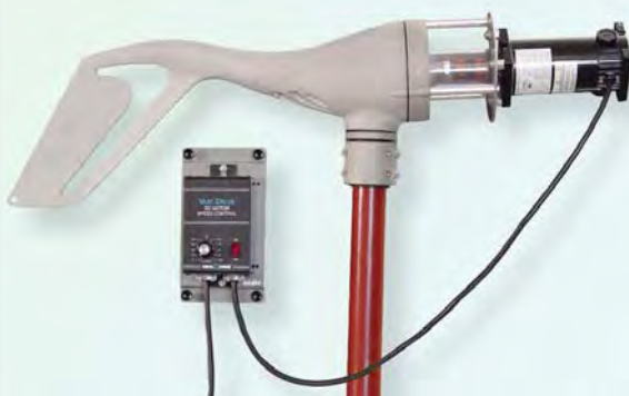
Wind Turbine Generator with DC Motor/ Controller (Wind Simulator)
